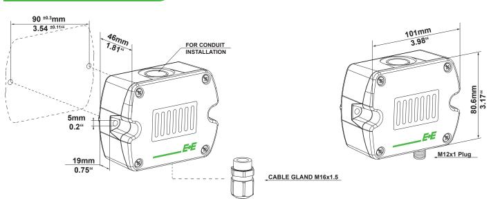
**EE820** with M12 plug does not require any wiring inside the device. The external mounting holes allow the device to be mounted without opening the front cover. The mating M12x1 cable plug for self assembly is included in the scope of supply. Please see EE820 data sheet for optional M12 plugs and cables.
