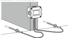
Use a Ø7.5 mm drill for installing the pressure connection nipples into the duct.
