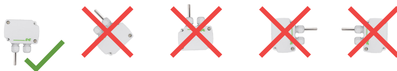
Fig. 5 Correct and incorrect mounting of the sensor
